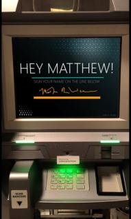
The pin number is validated, the customer is confirmed and the customer signs their name on the signature pad to accept payment. The camera at the top of the unit captures a picture of the customers face.
